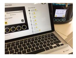
An image of the Braumeister controller is displayed. You can intervene in a controlled manner by starting a recipe, or manually, by turning the heater and pump on/off. Changing settings are made at the device manually and recipes are changed and developed with MySpeidel. In an emergency, the programme can also be stopped and terminated online.
