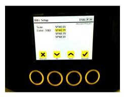
The requirement for using WIFI with MySpeidel.com is firmware version 1\_1\_27 or higher (the version number can be seen at the top right under *Settings*). Go to Settings and then click on WIFI.
