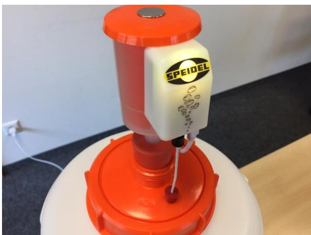
It is important that all passages into the fermenter are hermetically sealed and that fermentation gases can ONLY be discharged via the airlock. Connect the USB power cable to a power source and lay the cable so that moisture cannot run down the cable into the power supply. The LED should briefly light up in magenta and then switch to yellow (configuration mode).
