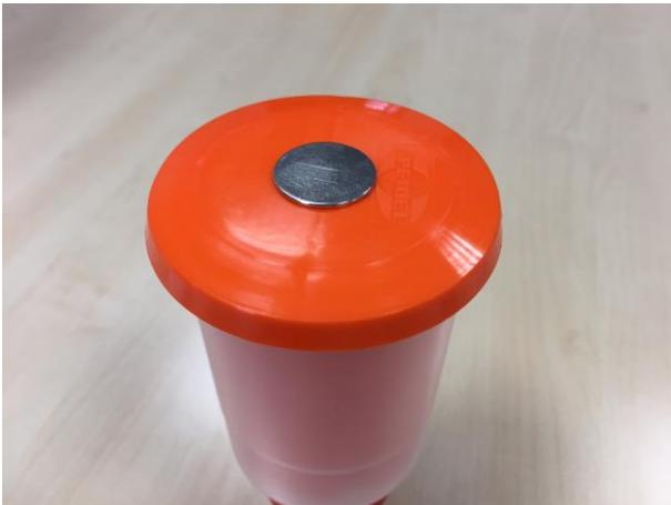
The adhesive magnet is centrally attached to the top of the orange airlock cover.
