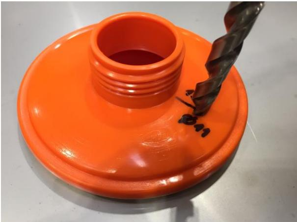
Using a suitable drill, a hole with a **10.5 mm** diameter (or with a 10mm drill, if a 10.5 mm is not available) is drilled into the cover of the fermenter directly below the sensor cable connection located on the attached airlock. We recommend a pre-drilling with a significantly smaller drill – particularly if the cover is made of stainless steel.
