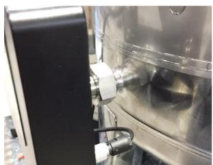
Push the Gärmeister with the temperature sensor rod all the way into the temperature sensor sleeve already pre-assembled on the tank and secure the horizontal position with the locking screw.
