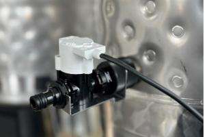
Connect the solenoid valve to a cooling unit if the circuit is to be used for cooling. Then connect the device to the power supply.
