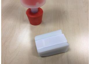
Stick the Velcro strip to the back of the module, pull off the adhesive strips and then stick the module in a vertical position onto the airlock directly below the upper edge.
