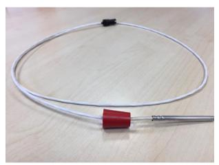
Afterwards, the sensor cable is inserted through the rubber plug or optional through an airlock rubber plug with additional whole (slightly dampen sensor and plug, so that it can be pushed through easier) and then the rubber plug is inserted very powerfully in a rotating motion so that the cable entry is firm and sealed. If necessary, pull the plug from the reverse side.
