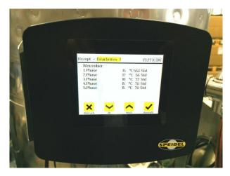
A fermentation recipe can be specifically named and it is possible to programme up to 5 phases with temperature and time in hours. Thus, fermentation or the yeast growth, for example, can be boosted with a higher fermentation temperature for e.g. 24 or 48 hours and the fermentation medium can then be lowered to an optimal fermentation temperature. Finally, prior to bottling after e.g. 200 hours, it is cooled back down to a low temperature in order to achieve an even better purification.
