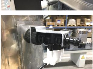
Insert the entire Gärmeister with the temperature sensor rod into the tank with the pre-assembled temperature sensor sleeve and secure the horizontal position with the rear safety screw.
