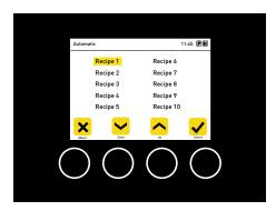
Go to the Start menu and press *Brewstart* and select the respective previously programmed and verified recipe. Start by pressing the *Select* button. Subsequently, the water starts filling. Follow the instructions in the program.
