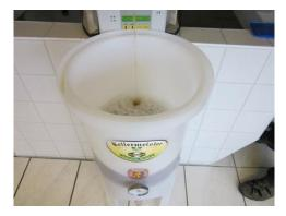
Pour the wort into a sterilized 12 L/ 30 L/ 60 L fermentation vessel. Use a disinfecting agent to clean the vessel and filling equipment. Settlements at the bottom of the vessel should not be filled. Add 11 g dry yeast to the wort and seal fermentation vessel by means of the fermentation lock filled with a disinfectant.
