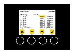
Plug in the Braumeister. The control is now in a basic state. In order to program a recipe, its time and temperature values, press the *Recipe* button. Use the arrow keys in the menu display above to select the recipe with which you would like to work. you can also create new recipes (up to 10) or delete recipes. Two standard recipes are included with the delivery. Press *Select* to invoke the recipe. Continue pressing *Select* while in the recipe step by step until you reach the end.
