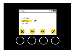
When pressing the *Settings* button in the main menu, the language, illumination, and time screen opens. The arrow keys allow you to make a selection, and choosing the *Select* function takes you to the various options. These, in turn, can also be selected by activating the arrow keys. Acknowledge your selection by pressing the *Select* button. Press the *Abort* button to return to the main menu.
